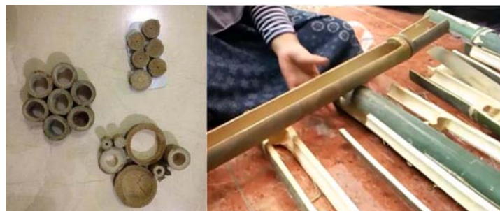
Figure 1. Widthwise cut and lengthwise cut of bamboo
